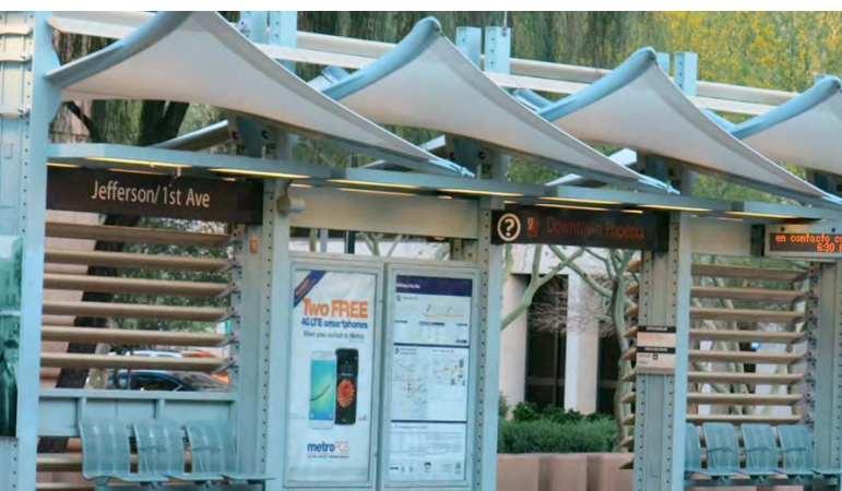
LEFT: The light rail station in Phoenix, Arizona, USA, provides shade using overhead canopies and slats that allow air to flow but protect users from the sun when the sun is low. Source: ITDP. RIGHT: Stations can be high quality public spaces that people enjoy. Weather protection and ample seating space encourage travel via public transport. Ahmedabad, India. Source: ITDP.
