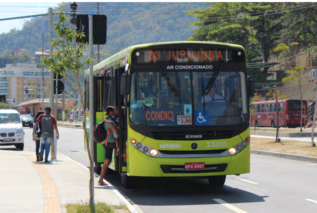
Lack of dedicated bus lanes or level boarding can significantly cause delays in trip times for everyone, but especially caregivers encumbered with goods and children. Niterói, Brazil. Source: ITDP
