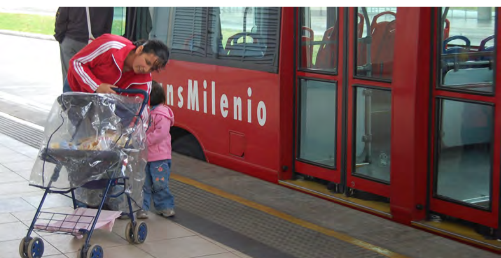
TransMilenio, the BRT system in Bogotá, Colombia, has level boarding and off-board fare collection as part of its system design, which helps caregivers use the system. Source: Carlos Felipe Pardo.
