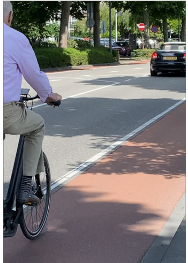
Image:267 Colored asphalt cycle track
